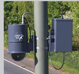
The third system available from Swift is the Swift Streetcam, which has the added advantage of being semi-covert with installation occurring in the standard Phillips street light fitting. The system can easily be integrated with an existing CCTV control room and is simple to deploy requiring only street lighting personnel. The system allows real time transmission and can utilise licensed and unlicensed frequencies. The receiver unit can be covertly positioned up to 2km away from the camera.
